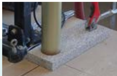
Trockenbohren in Granit
