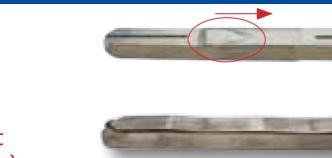
**Step B:** Insert template onto the spindle and position it, using the millimeter indication on it. **(Please note the sizes of different countries as they change according to the country's standards).** Align and centre mark the hole position .
