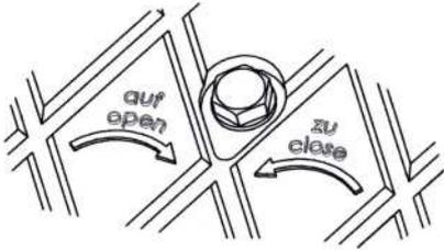
Turning the hexagonal head of the screw on the top of the lid (B) opens and closes the safety latch. The latch locks into a slot or into the inner edge of the inspection chamber. (Point 2.2.1)
