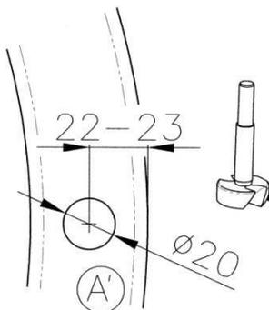
With inspection chamber directly on the tank, the drilled hole for the locking bolt is aligned to the cover. If this needs adjusting, an additional drilling of A can be made, see figure on the left.
