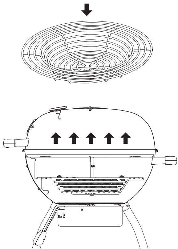
For this cooking method, the lid can be left open or removed if necessary. To do so – when the appliance is cold – remove the split-pin from the lid hinge and then pull the hinge pin out of the two halves of the hinge. Then refit the split-pin in the hinge pin and store the lid in a safe place.
